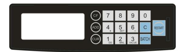
**CF (counterfeit detection):** press it to turn off/on UV, MG, MT, IR detection. **ADD:** press this button to turn on/off the ADD function.
