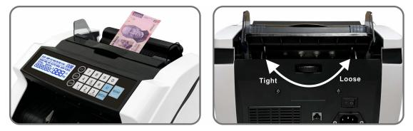
When banknote feeding is unsmooth or banknote counting is inaccurate, it can be solved through adjusting the vertical adjusting screw as well as the gap between resistance rubber and rubber wheel. Then you can put in a banknote and hold, if you feel the pull, the machine is workable.
